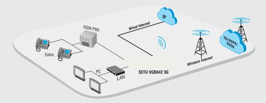
Furthermore, it provides fail-over connectivity by automatically routing all VoIP calls and data traffic over UMTS (3G) network in case of wired internet connectivity outage.
